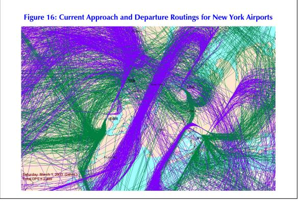
This representation is a recording of actual flight tracks on one day in 2003. The complexity of this interlacing of arriving and departing aircraft at all the New York-area airports is a major cause of delays. (Source: Port Authority of New York and New Jersey)
