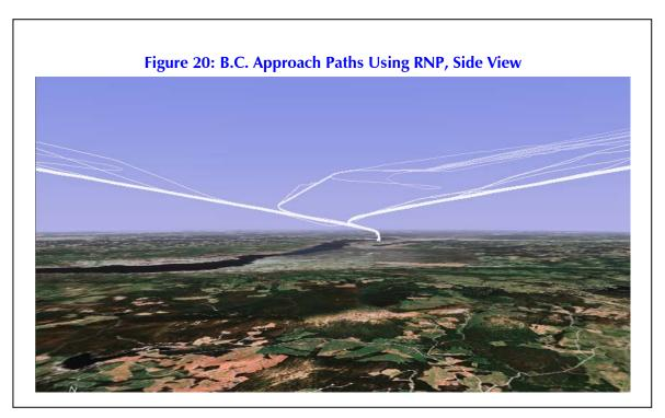
Side view of the same approach paths after the RNP Approach System is implemented. The same results can be achieved in New York with a resulting flow of single lines replacing the many different lines shown in Figure 19. (Source: Naverus Corp.)
