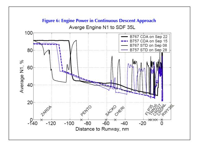
Comparison of continuous vs. standard descent engine power changes on approach, showing the significant reduction of engine power settings, providing a much smoother approach that reduces noise and provides other benefits. (Source: Bob Hilb UPS Airlines)
