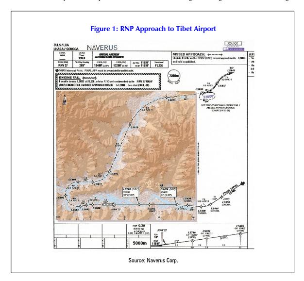
This map shows the routing of an aircraft through 20,000 foot mountain canyons to land at Lhasa, Tibet. The routing is flown automatically, by RNP methods, in bad weather. This ability can be
