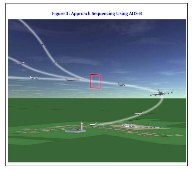
Continuous Descent Approaches combined with automatic sequencing using NextGen technologies bring various size and speed aircraft to final approach separated for wake turbulence, speed or any other desired criteria. (Source FAA)
