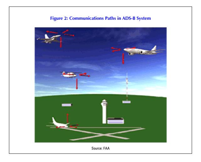
This rendering depicts the multiple paths of communication used by ADS-B systems. Each aircraft knows where all other aircraft are and where they are headed. The ground has a complete picture of where the aircraft are, where each is going and how they interact.
