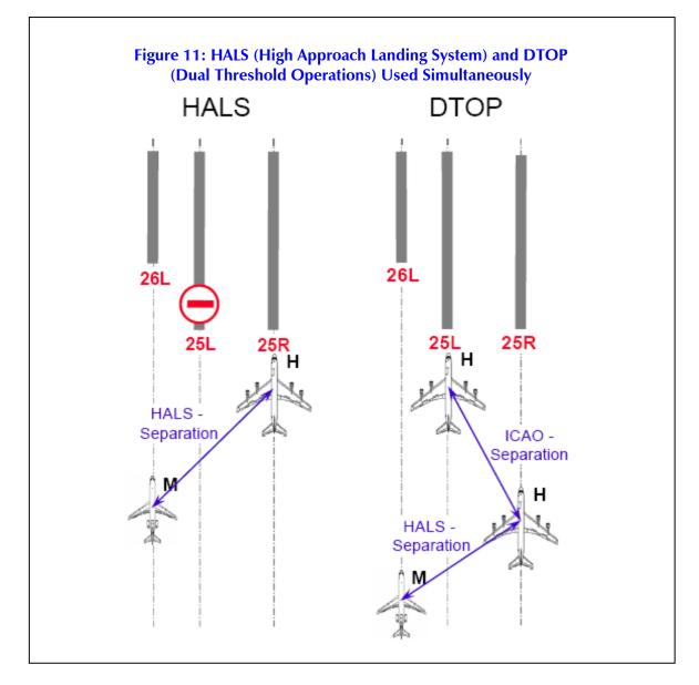
The aircraft on the left is flying higher than the others and can thus fly closer behind the others. H stands for heavy jet and M stands for medium jet. (Source: Frankfurt Airport Capacity Enhancement Program the Role of Wake Vortex Reducing Measures 2nd WakeNet 2 - Europe Workshop, 30.11. – 01.12.2004)
