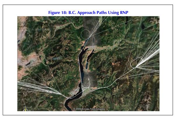
This figure shows the precise and repetitive nature of this new technology. Every aircraft follows the same path all day long. These paths can be designed to follow any routing. (Source: Naverus Corp.)
