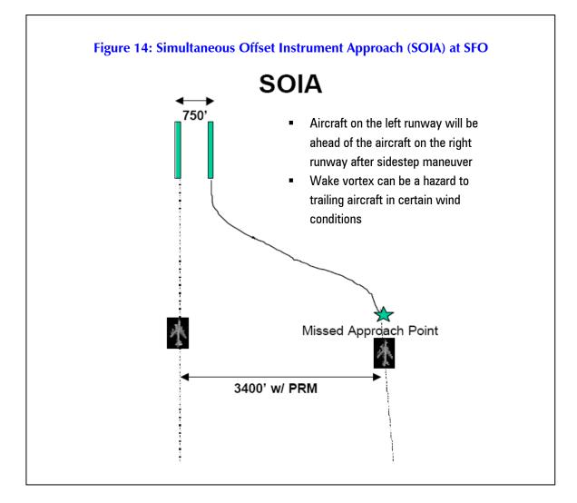
This figure shows the approaching aircraft on the right maintaining a path 3,400 feet or more separated from the left aircraft until the aircraft can maintain visual separation below clouds after the missed approach point indicated by the green star. (Source: FAA)
