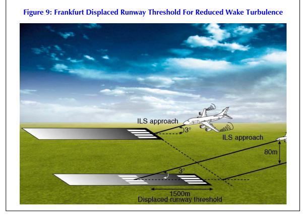
This shows that if a smaller jet flies on a higher approach path that lands farther down the runway it is not affected by wake turbulence from the larger jet. (Source: Bram Elsenaar, WakeNet2-Europe).
