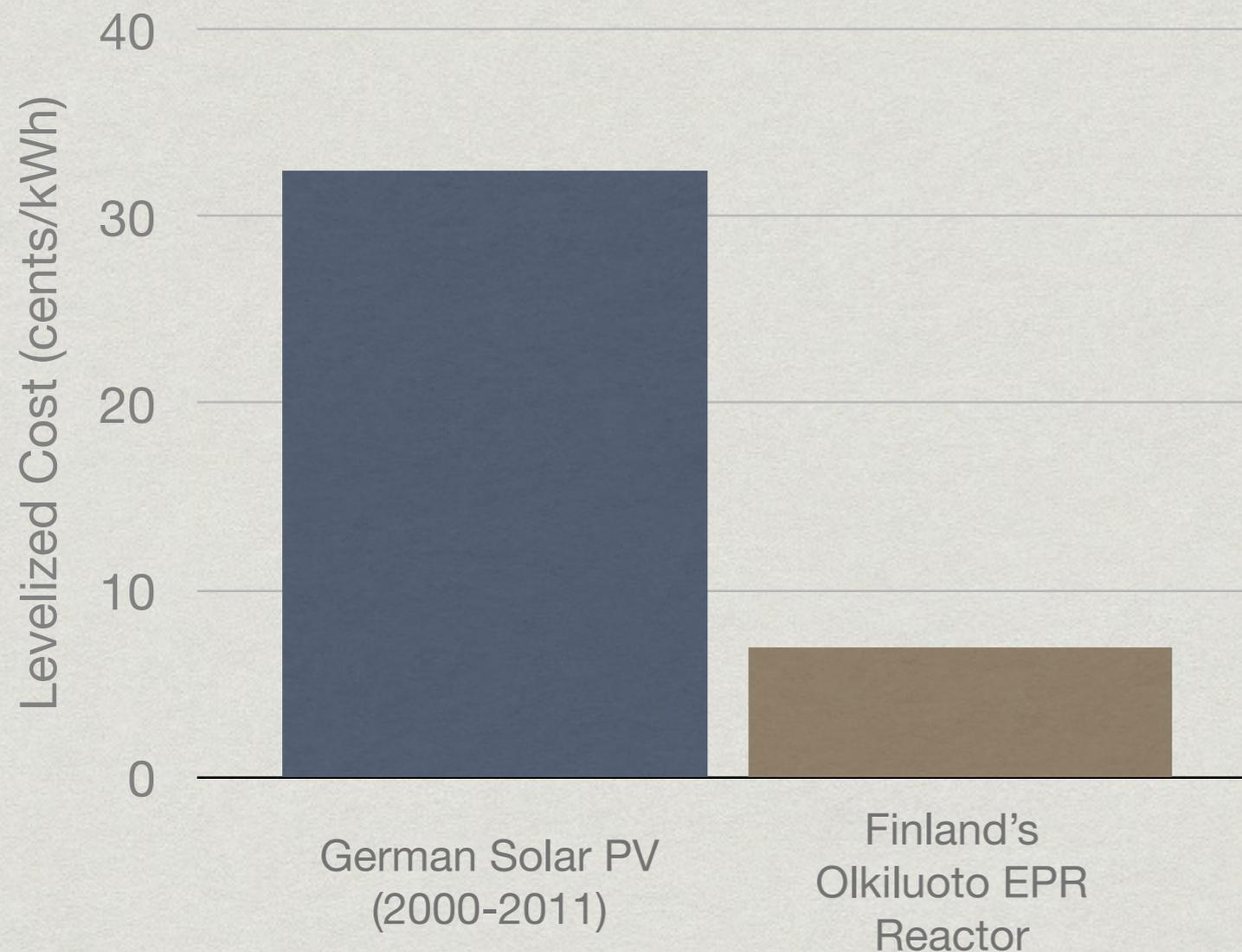
The German solar program is lauded as a great success, while the Finnish EPR is derided as proof that nuclear is doomed. Yet, when looking at the levelized cost to produce electricity, German solar is **four times** the price of the over-budget Finnish nuclear plant.
