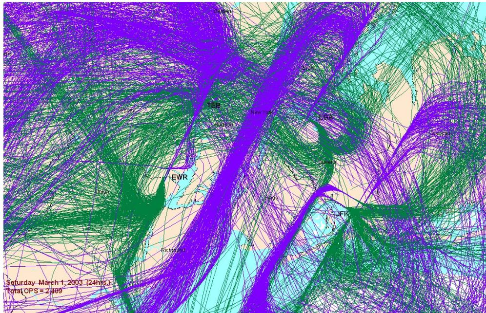
*This representation is a recording of actual flight tracks on one day in 2003. The complexity of this interlacing of arriving and departing aircraft at all the New York-area airports is a major cause of delays. (Source: Port Authority of New York and New Jersey)*
