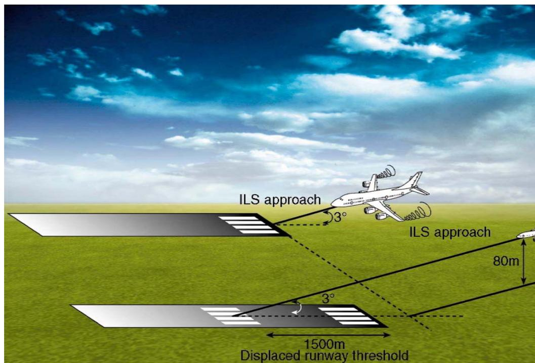
*This shows that if a smaller jet flies on a higher approach path that lands farther down the runway it is not affected by wake turbulence from the larger jet. (Source: Bram Elsenaar, WakeNet2-Europe).*
