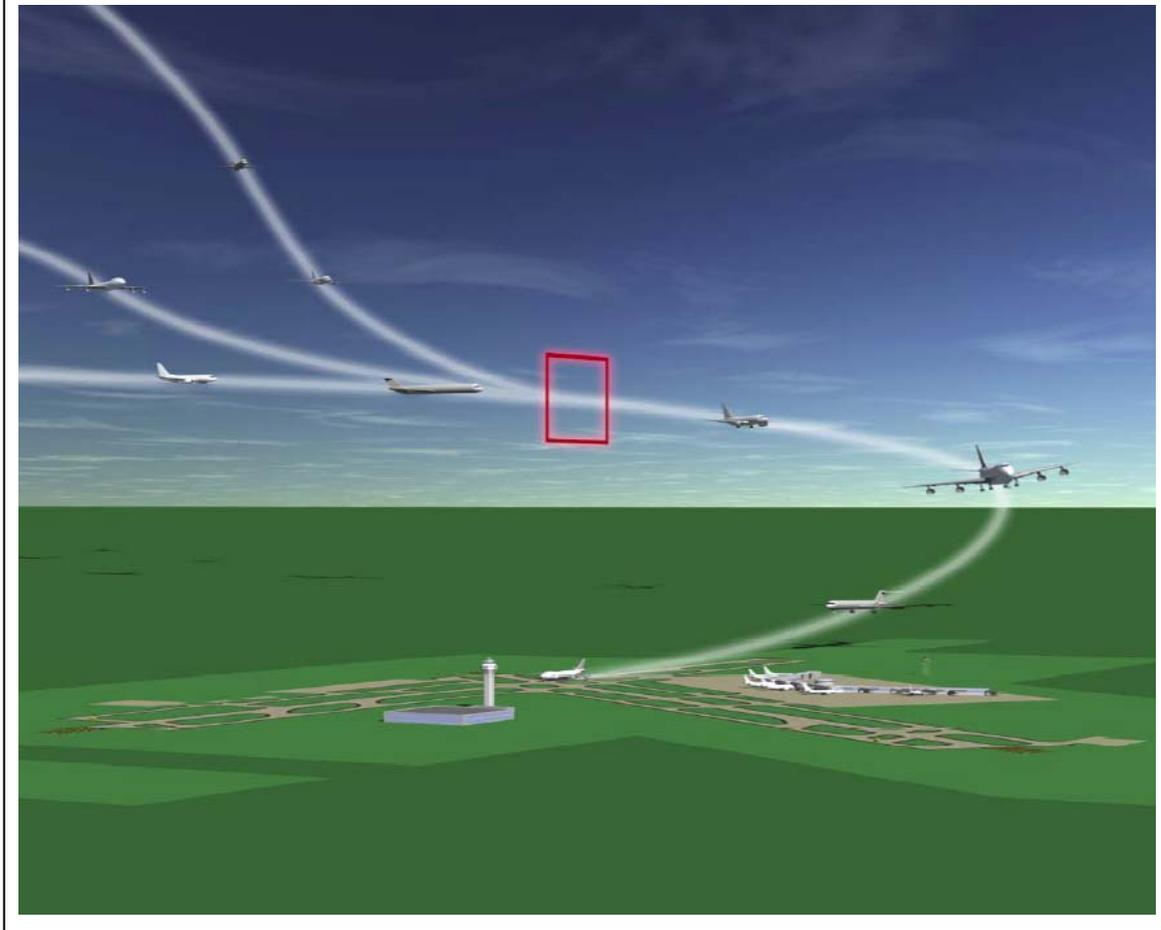
*Continuous Descent Approaches combined with automatic sequencing using NextGen technologies bring various size and speed aircraft to final approach separated for wake turbulence, speed or any other desired criteria. (Source FAA)*
