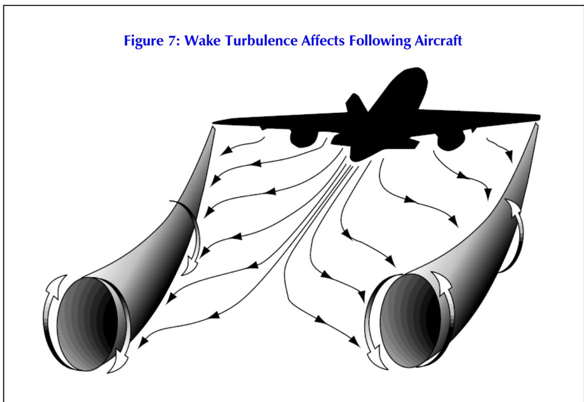
*The picture reveals the expanding outward impact of disrupted air that trails behind a large aircraft and disrupts the stability of a following aircraft. (Source: FAA)*
