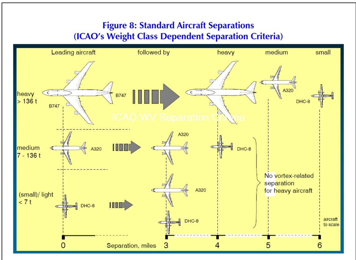
*Separation distances between various aircraft as currently applied. The top row shows the following distances behind a large jet for a medium jet and a commuter airplane. For example an A320 needs to follow a 747 by five miles. The center and lower rows show the same for small jets and aircraft. (Source: Bram Elsenaar, WakeNet2-Europe)*
