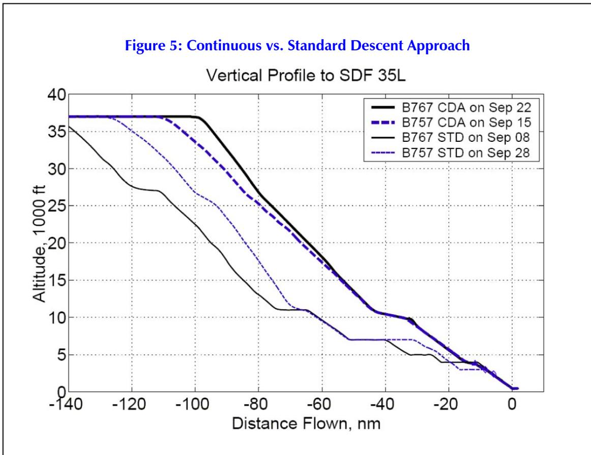
*Comparison of continuous vs. standard descent altitude changes on approach, showing the lack of changes in altitude settings. (Source: Bob Hilb, UPS Airlines)*
