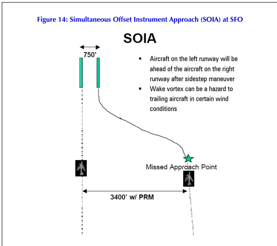
*This figure shows the approaching aircraft on the right maintaining a path 3,400 feet or more separated from the left aircraft until the aircraft can maintain visual separation below clouds after the missed approach point indicated by the green star. (Source: FAA)*
