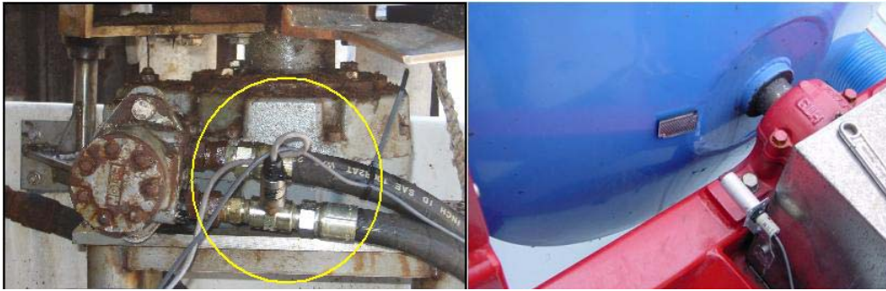
Figure A4 A hydraulic pressure sensor installed on the supply line of a vessel line hauler (left). Drum rotation sensor (right) mounted on pelagic longline vessel, showing optical sensor and reflective surface.
