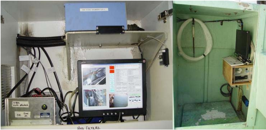
Figure A1. EM control box and user interface installations on two different vessels.
